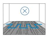
4. For a natural look, we recommend that the piece left over from the first row should not be used as the first piece of the second row. Avoid having a recognisable, repeating distance between the panels, which creates a kind of staircase effect. Boards are installed randomly and tiles can be installed in a straight line, in a half-brick bond or in an irregular bond.
